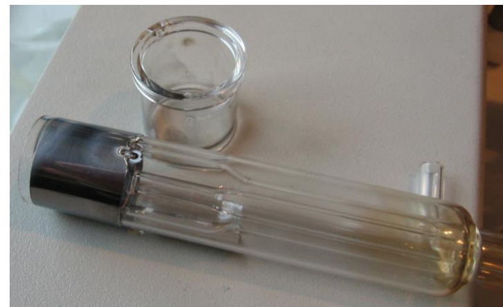
Torch damage due to incomplete drying
