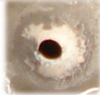
Close up of sampler cone after measuring 75 undiluted sea water samples using HMI
