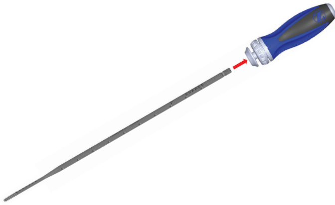
Figure 18 Tap and ratcheting handle assembly
