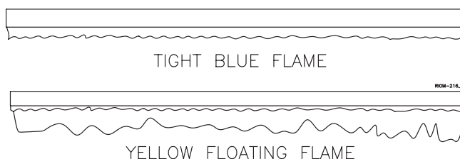
Figure 20 - Main Burner Flame
