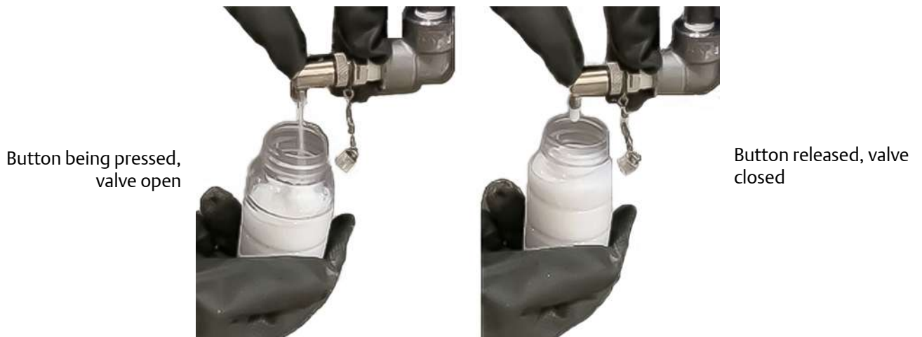
Figure 5-5. Operating the Oil Sampling Valve
