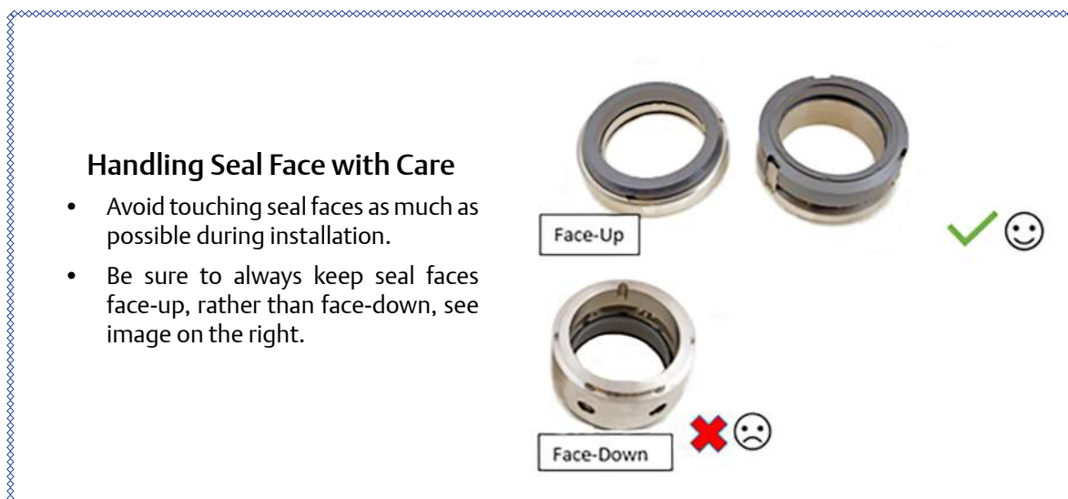
Figure 5-59. Handling Seal Face with Care
