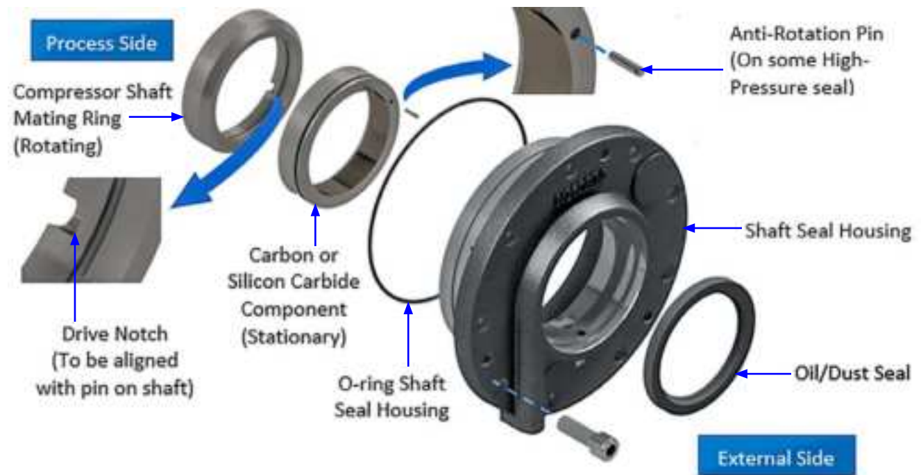
Figure 5-58. Shaft Seal Assembly
