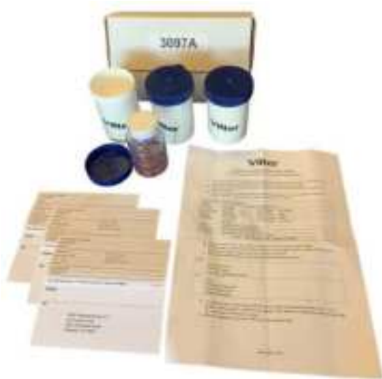
Figure 5-2. Oil Analysis Kit (VPN 3097A)
