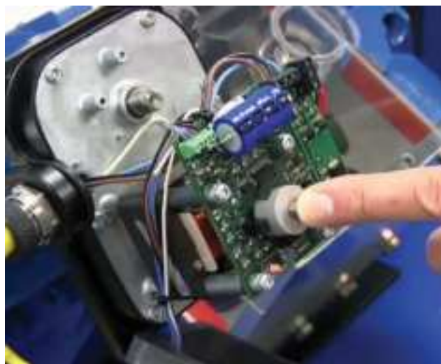
Figure 4-10. Photo-chopper Press down on Photo-chopper to release tension from motor shaft.
