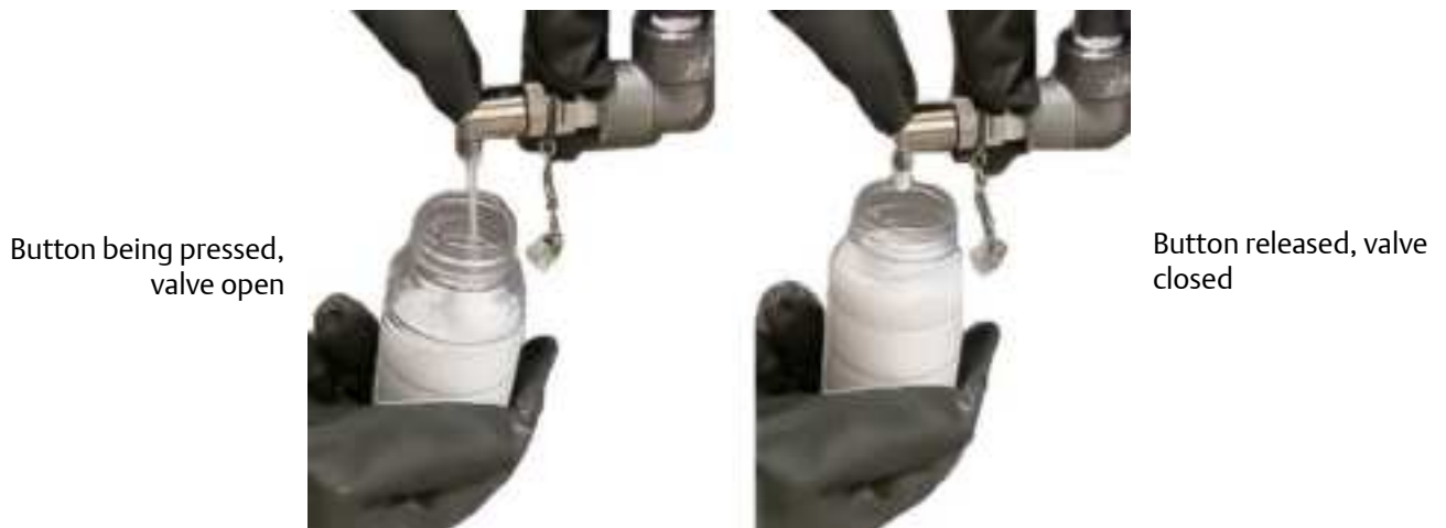
Figure 5-5. Operating the Oil Sampling Valve
