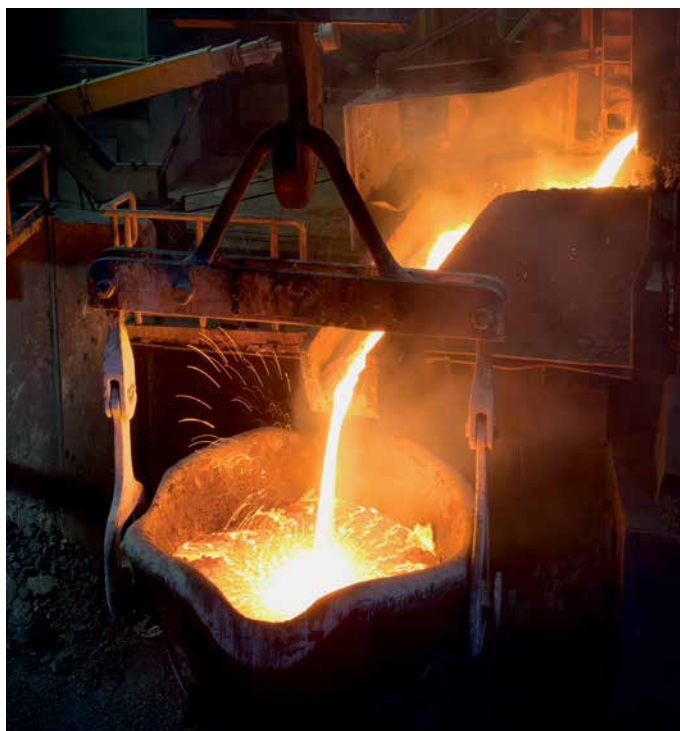
High temperatures: Liquid copper matte flows out of a flame furnace.
