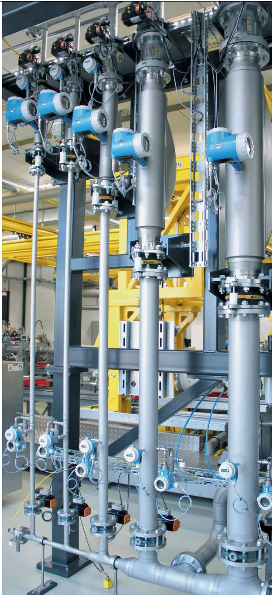
Ex-works precision: Endress+Hauser can calibrate flowmeters with hydrocarbons on request.
