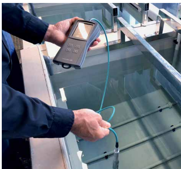
Easy to use: The new Teqwave T measures liquid concentrations in the passivation bath.
