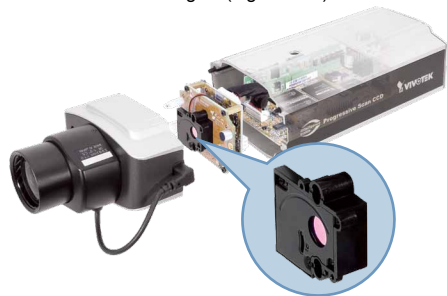
Figure 2.16 Placement of ICR
