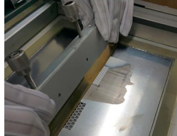
Place the squeegee or spatula behind the TIM and tilt down it to have 45° angle around. Apply a certain pressure and draw the squeegee downwards slowly.
