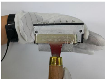
Figure 13. Example of Thermal Paste Application Using a Rubber Roller
