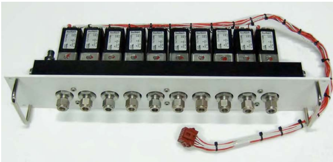
Figure 5. 10 Sample valve manifold
