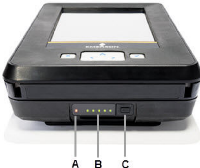
Figure 2-9: LEDs showing approximately 100 percent charge
