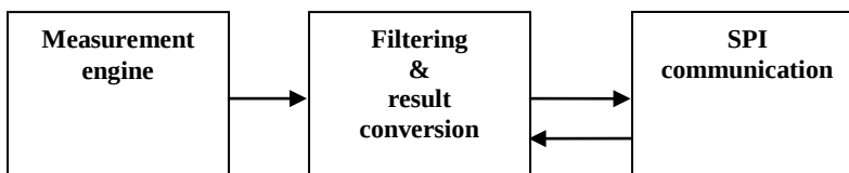
Figure 2. Block diagram of the data acquisition firmware
