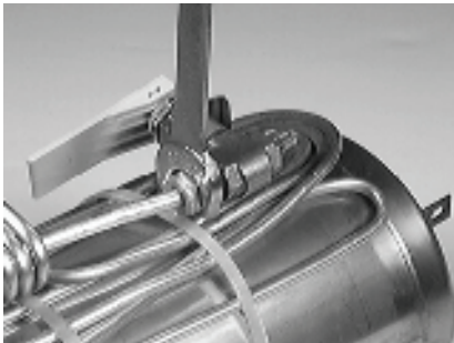
Figure 20: Vent Tube Removal
