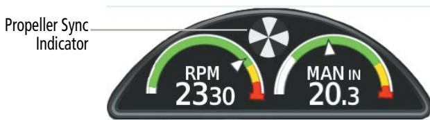
Propeller Sync Indicator Example
