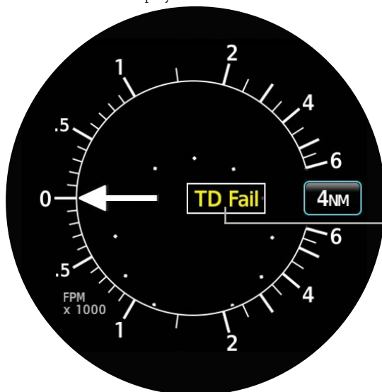
TD Failure Annunciations
