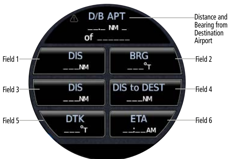
'MFD Data' Page (Flight Plan Information Received from External Source)
