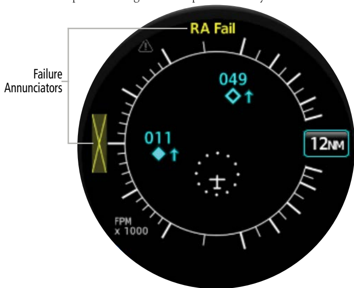
RA Failure Annunciations
