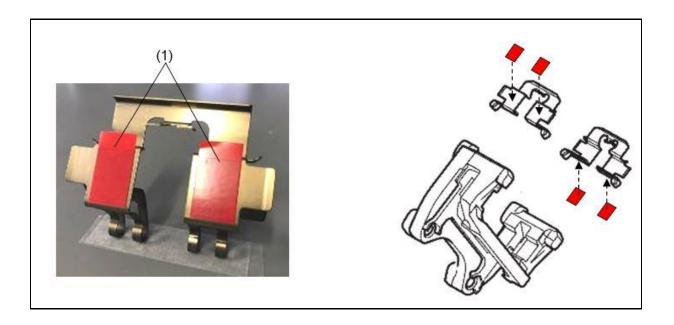
4. Peel off the red release film from the dual adhesive tape.
