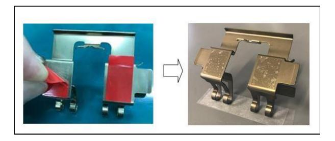
5. Reinstall the guide plates to both mounting supports.
