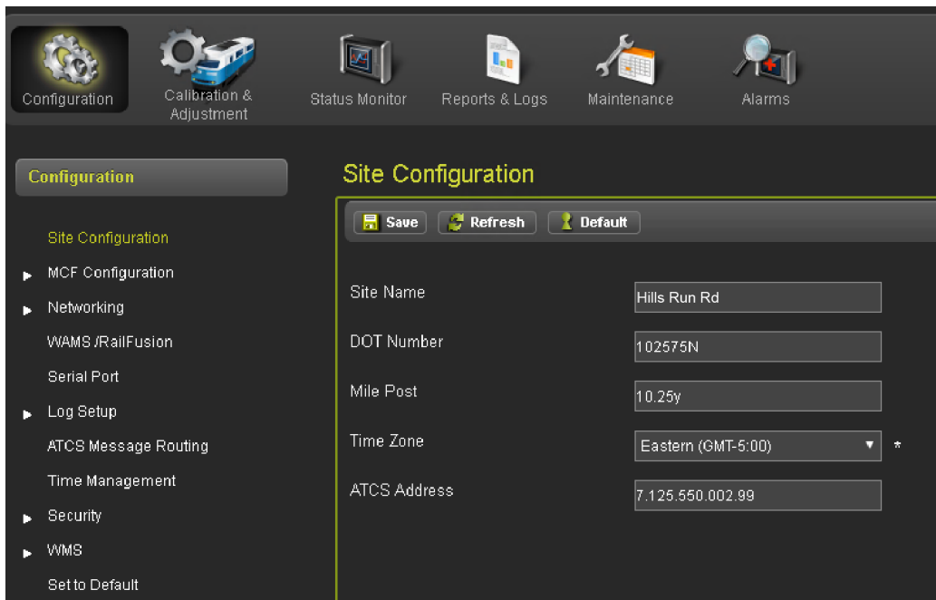
Figure 5-5 Site Configuration Screen
