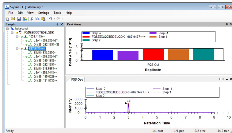
Figure 6 Comparing collision energies for the same transition
