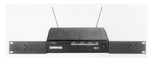
RACK-MOUNTING SINGLE UNIT WITH WA500 MONTAGE D'UNE SEULE UNITÉ AVEC WA500 EMFANGER EINZELMONTAGE MIT WA500 MONTAJE DE UNIDAD ÚNICA CON WA500 MONTAGGIO AD UNITÀ SINGOLA CON WA500
