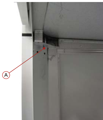
Figure 3.10 A: M8 screw seen from underneath.
