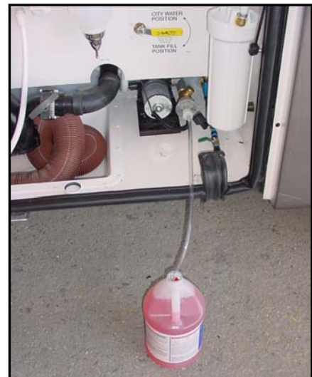
Figure 14-17. Wintering Process for the Motor Home
