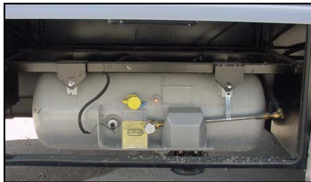
Figure 3-4. Liquid Propane Tank
