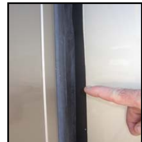
Figure 14-5. Inspecting Slide Out Gasket
