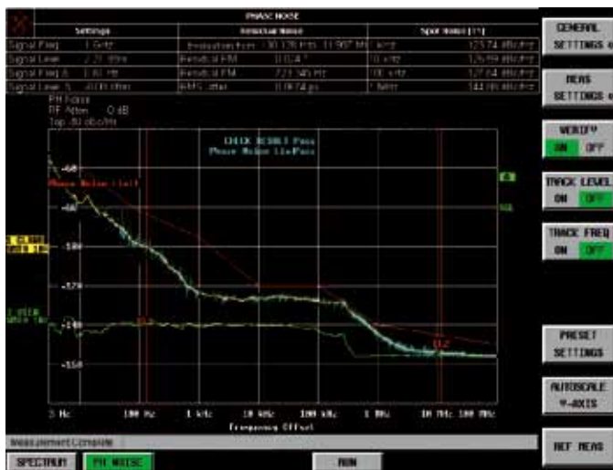
Phase noise measurement using the R&S®FS-K40 application firmware.
