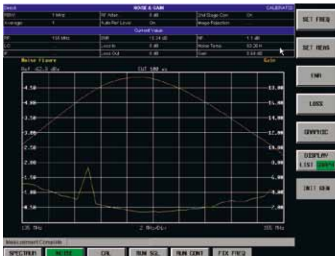
Noise figure measurement using the R&S®FS-K30 application firmware.
