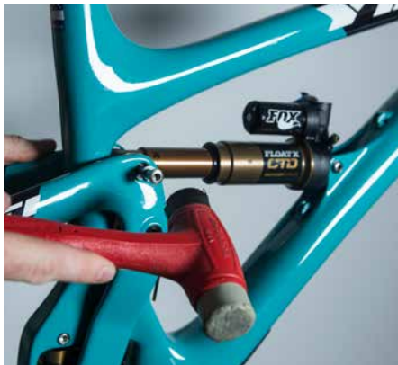
13. Using a soft mallet push the female shock mounting hardware through the frame and shock on the Fox Guide Pins.
