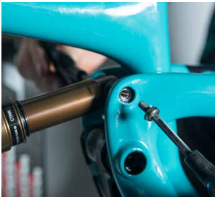
14. Prep and install the male shock mounting hardware on both ends of the shock. Apply Blue Loctite (248) to the threads and install the washer. Thread the bolt in snug, but do not torque.
