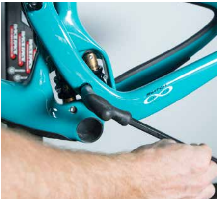
16. Using a 10mm allen wrench finish tightening the main pivot axle and the upper link axle. Torque the pivot axles using a properly calibrated torque wrench.
