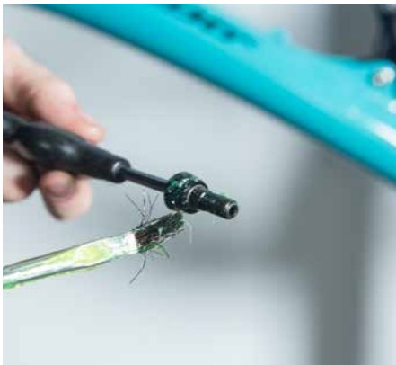
17. Prepare both your collet bolts with grease. You want to have grease on the threads and on the collet wedge.
