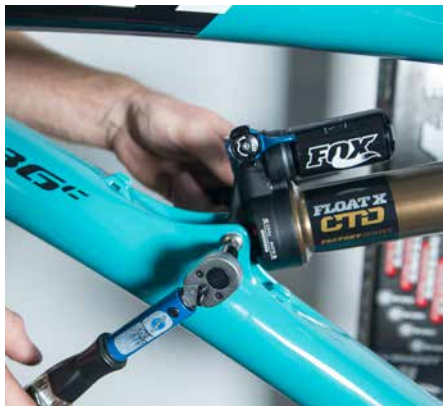
15. Time to get the torque wrench out. Using a 5mm allen on one side and your properly calibrated torque wrench on the other torque the shock mounting hardware on both ends of the shock.
