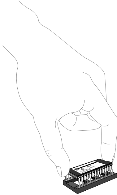
FIGURE I-6. Inserting the New PROM
