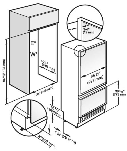
E\*: The position of the electrical connection should not be higher than 9" from the floor.
