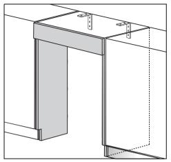
screw the cabinet to the wall behind it in several places using suitable mounting brackets.
