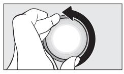
Turn the light cover counterclockwise and pull out.
