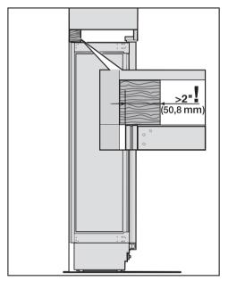
If possible, always screw the wooden beam to existing studs.
