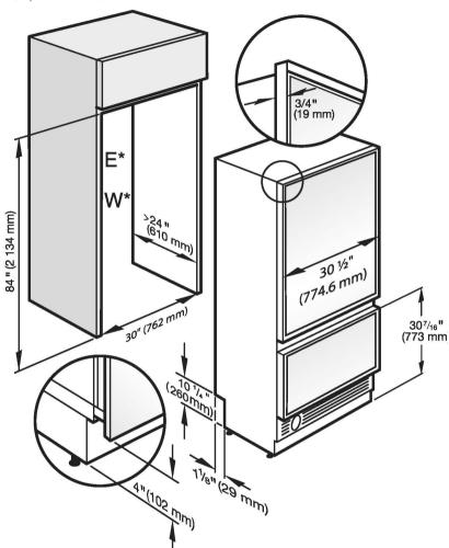
E\*: The position of the electrical connection should not be higher than 9" from the floor.
