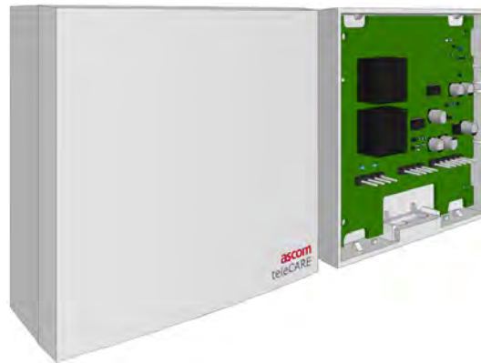
Figure 233. Television interface module: front and back view
