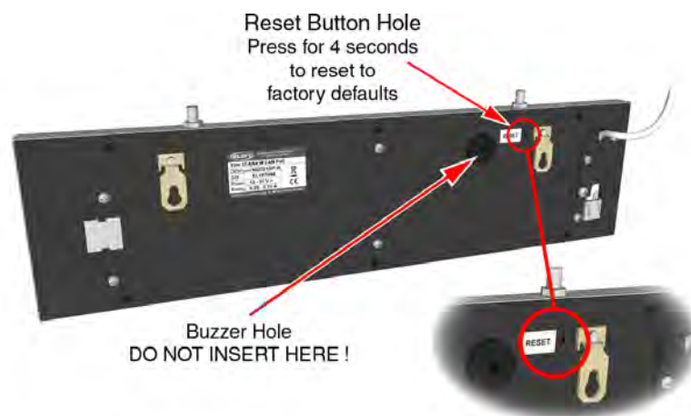
Figure 306. Reset button hole on the NUCD12IP-H
