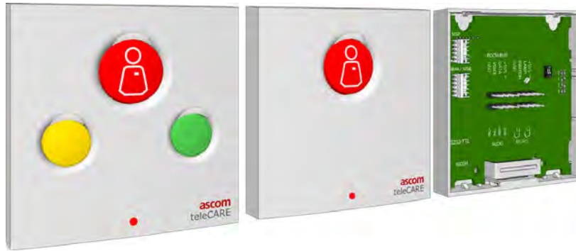
Figure 270. Bedside module NIBM2: front and back view
