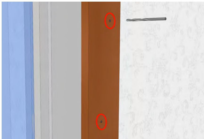
Figure 383. Drill the two holes with the proper drill
