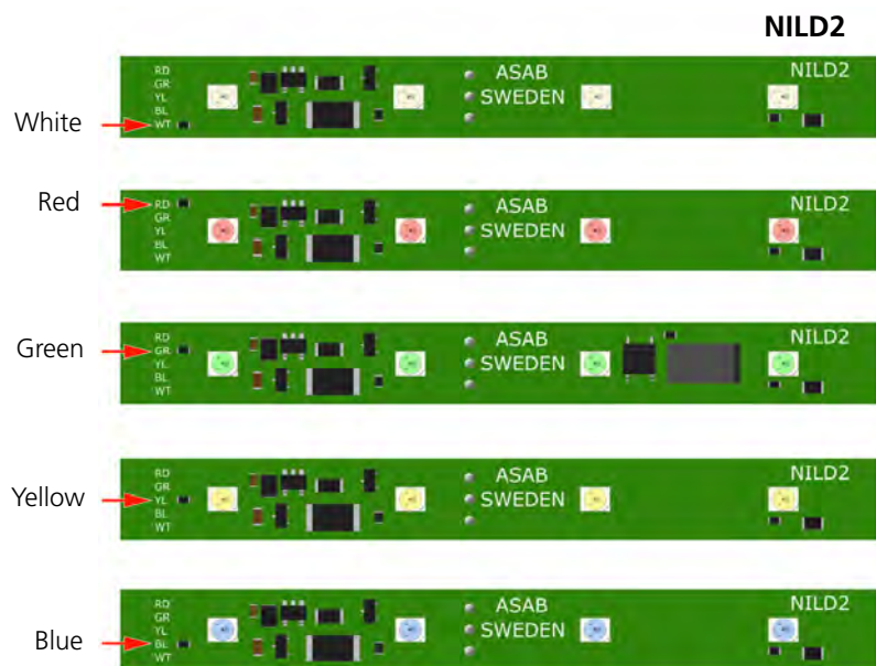
Figure 75. NILD2 - LED lamp boards: white, red, green, yellow and blue
