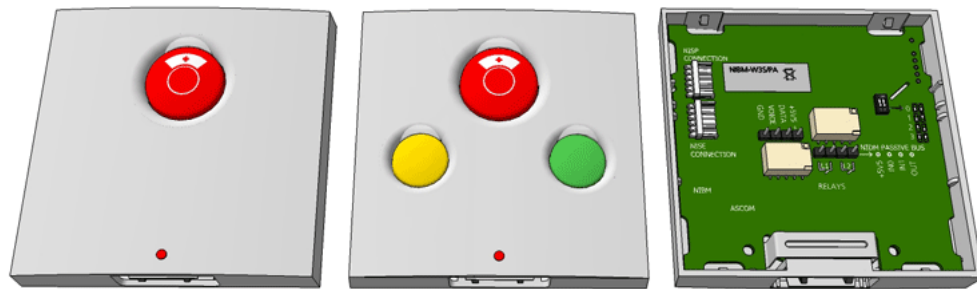
Figure 156. Bedside module NIBM - 1 button and 3 button front and back view
