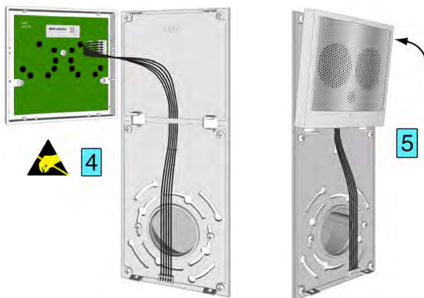
Figure 230. Connecting the NISP and mounting it on the backplate
