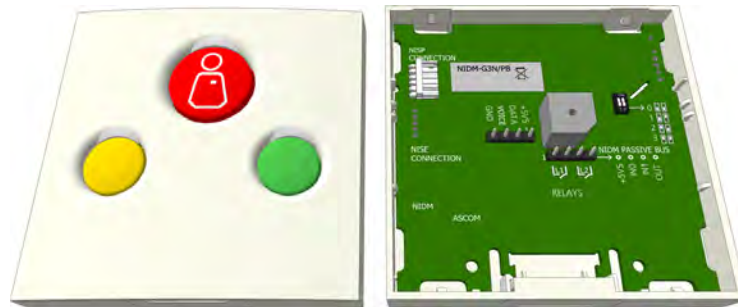
Figure 176. Doorside module: front and back view
