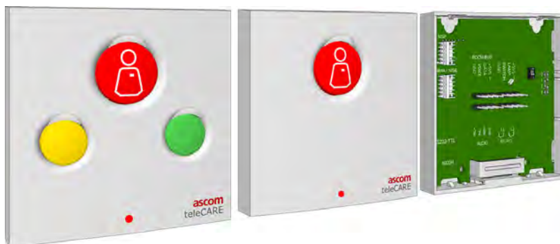
Figure 152. Bedside module NIBM2: front and back view
