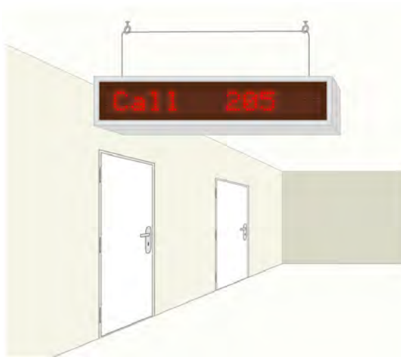
Figure 285. Ceiling mounted corridor display
