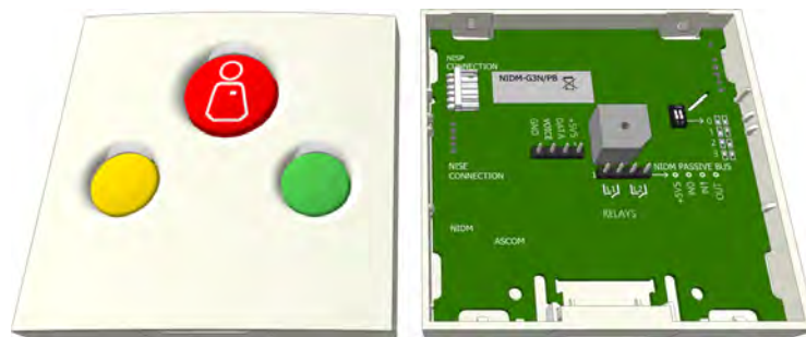
Figure 271. Door side module: front and back view
