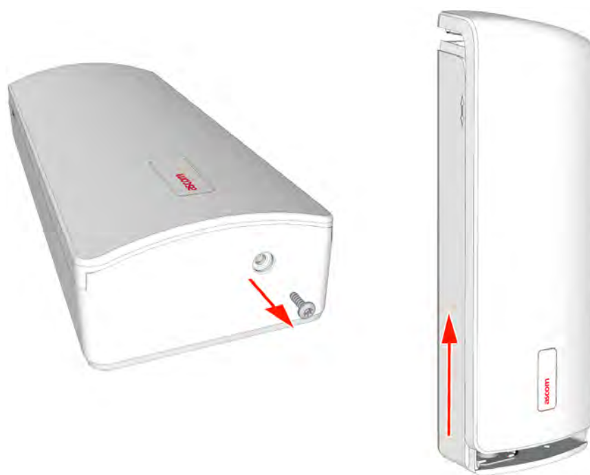
Figure 381. Removing the front cover of the NILF
