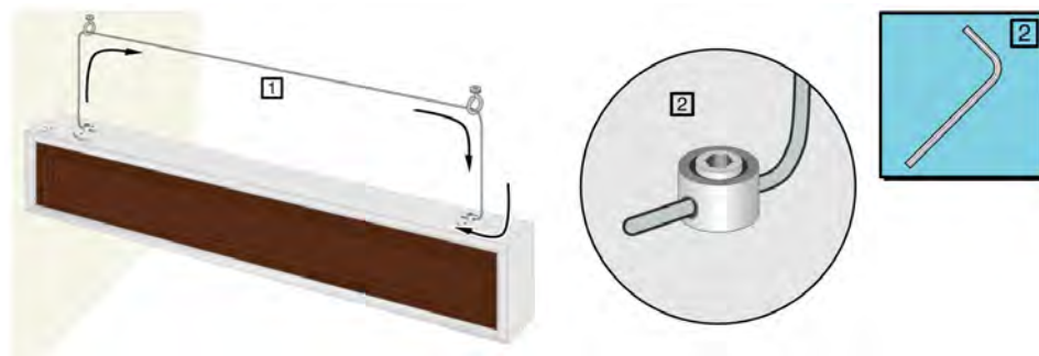
Figure 301. Close the loop and tighten the suspension wire
