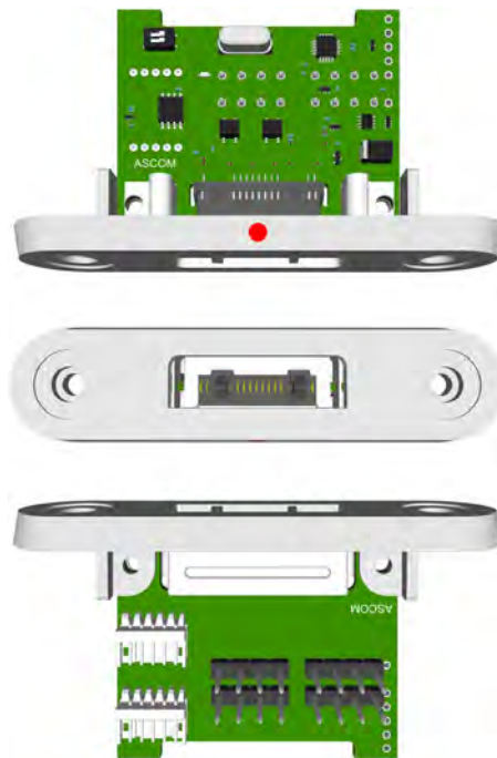
Figure 166. Medical Rail Module NIMS2 (top, front, bottom)
