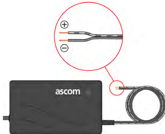
Figure 12. 24V/4.2A power supply unit output wires polarity
