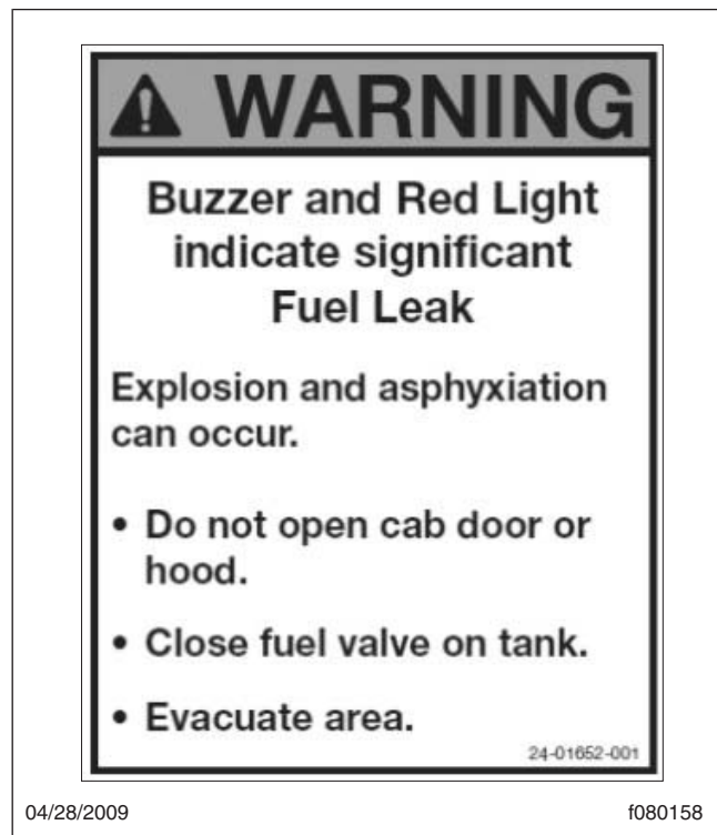
Fig. 25.5, Exterior Warning Sticker
