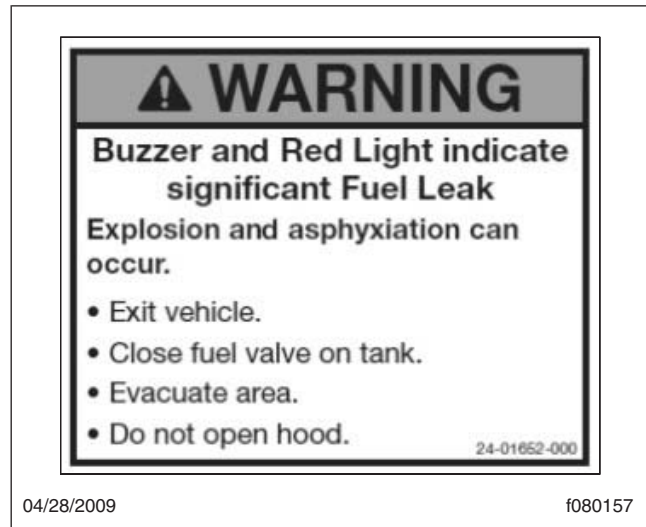
Fig. 25.4, Interior Warning Sticker
