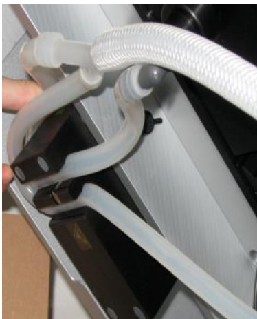
Hose exiting from the pinch valve.
