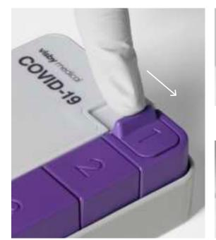
▲ After loading sample into device, close Button 1 by **sliding** the cap to the right.
