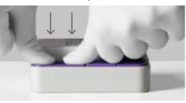
Push Button 3 all the way down. Use two thumbs, push firmly. Note: All buttons should be all the way down.
