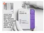
Plug in the device until it clicks into place. A stable white light indicates the test is running.
