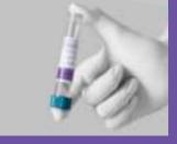
C Open the cap of the Visby Buffer Tube. Place cap wet-side up. Take the tube 5 times. the Visby pastette
