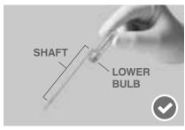
**G** Fill the **entire shaft** with fluid. Some fluid should enter the lower bulb.
