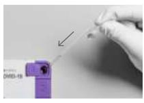
Place the tip of the pastette into Sample Port (Button 1). Squeeze the bulb to dispense the liquid. Some fluid will remain in the lower bulb.
