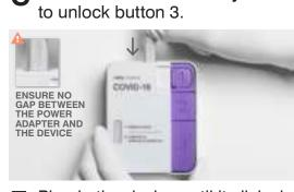
Plug in the device until it clicks into place. A stable white light indicates the test is running.
