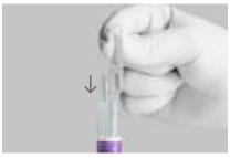
**E** Keeping the bulb squeezed, lower the pastette tip to the bottom of the Visby Buffer Tube.
