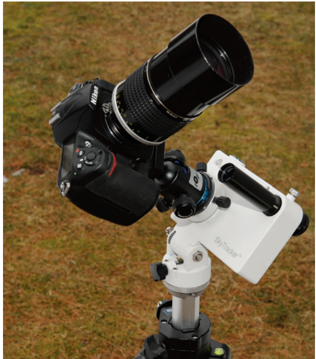
The author tested the SkyTracker with it attached directly to the center column of a heavy-duty Manfrotto tripod. If the polar-alignment scope interferes with equipment mounted on the tracker, it can be removed after the tracker is aligned.
