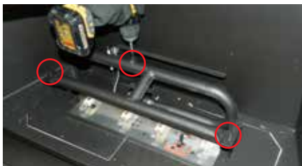
Diagram 2: Slide burner assembly to the right—then remove.
