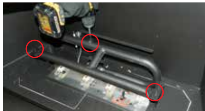
Diagram 2: Slide burner assembly to the right—then remove.
