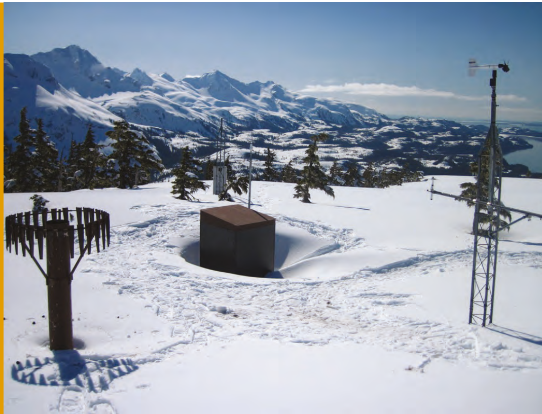
Example of a typical SNOTEL site. Image: USDA Natural Resources Conservation Service
