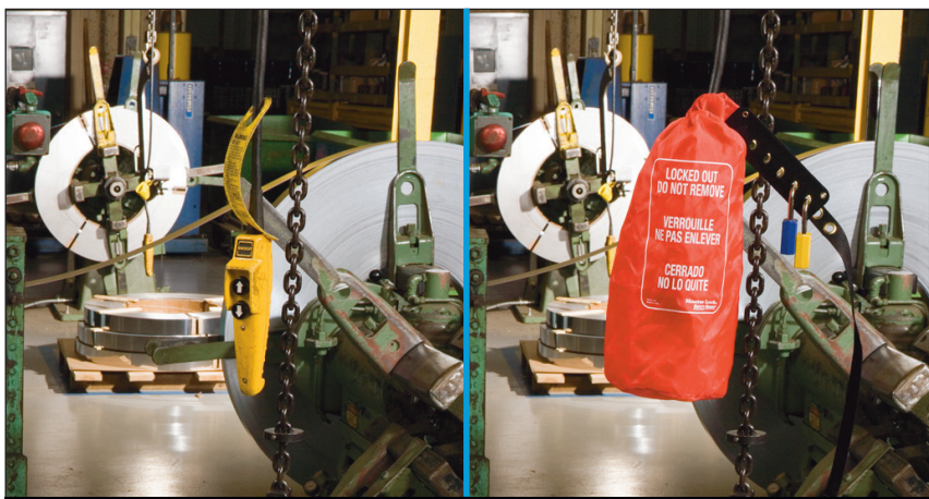
Hoist Control Cover
