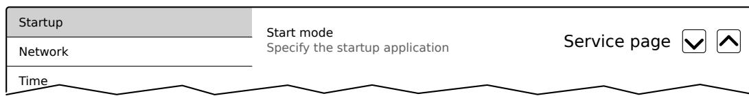
The start mode is configured the service page *Startup* and determines how the Power Panel behaves after being switched on. The Power Panel is started in one of the following modes (*Start mode*) in accordance with this setting:
