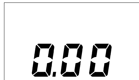
First press on timer button starts 10 minute countdown
