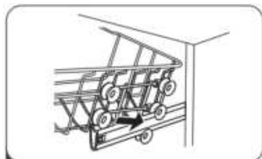
3 Re-attach the upper basket to upper or lower rollers.
