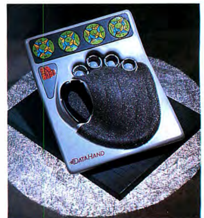
The DataHand is an alternative keyboard under development by Industrial Innovations.
