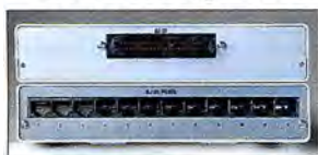
Every hub ships with interchangeable back panels that allow you to connect using either RJ-45 jacks or a 50-pin connector.
