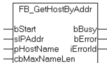
Fig. 83: Function block FB_GetHostByAddr
