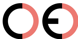
False CE Mark (too far)
