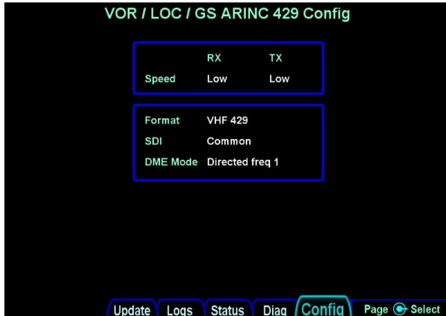
Figure 20 VOR/LOC ARINC 429 Configuration Page
