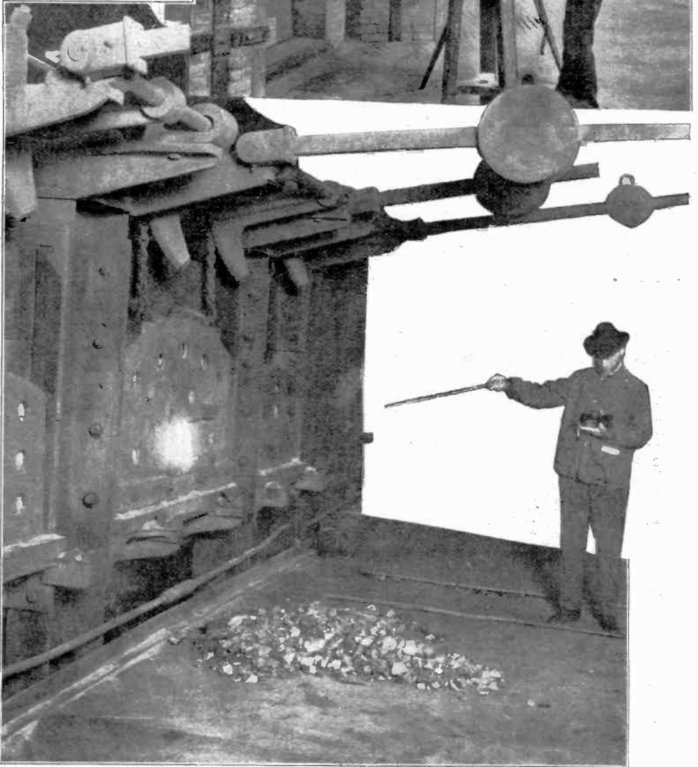
PORTABLE RADIATION PYROMETER, DESIGNED BY CHARLES BURTON THWING—DETERMINING THE TEMPERATURE IN AN OPEN HEARTH STEEL FURNACE
