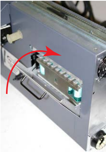
Analyzer Filter Door
