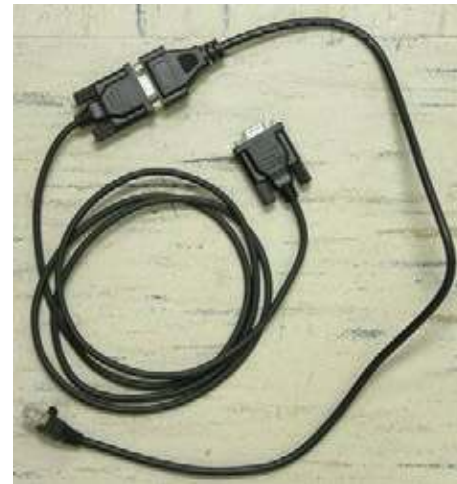
Figure F-5 -- Debugging Cable
