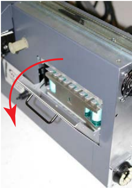
Analyzer Filter Door
