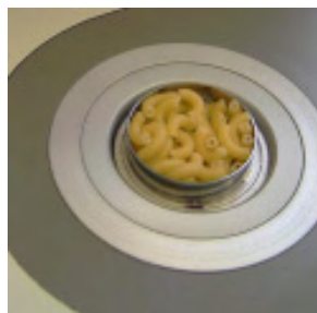
Place the probe inside the basket over the SAL-T into the measurement chamber
