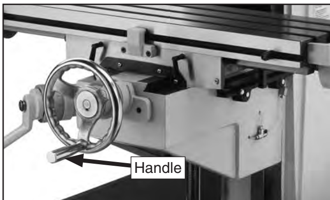
Figure 12. Cross feed handle attached to handwheel.
