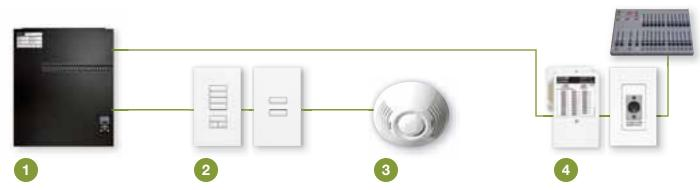
LCP128 SpecGrade panels and integral programmer provide architectural dimming control and programming capability for up to 500 events and up to 128 fullyrated 16A lighting zones.
