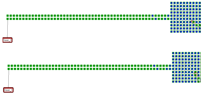
Figure 7-5: Component Test 14(ii) where the stretcher has displaced four agents in a 30° orientation and five agents in a 65° orientation
