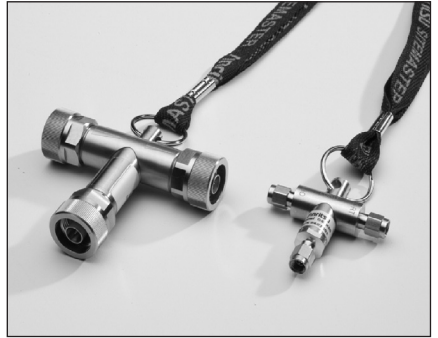
Figure 11. Convenient calibration components for the VNA provide the Open, Short and Load standards for the SOLT calibration procedure.
