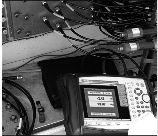
Figure 9-9. In contrast to a bulky VVM system with power cords, the portable network analyzer moves in close to the test cables and antennas to streamline installation and maintenance of systems.
