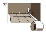
• The diagrams below indicate where the Harmonics® planks are clicked together by angling up and down or where they are tapped together flat. Follow the diagrams precisely. (See diagrams 4.1 through 4.16.)
