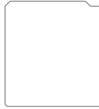
End Cover Plate Fastened at the opening of the last Plenum in the "line-up" opposite the exhaust end to seal Plenum end
