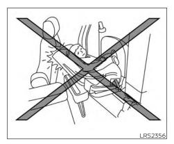
The front seat cannot be used when a rear-facing child restraint is installed on the jump seat. Attempting to do so could cause serious injury in a sudden stop or collision.
