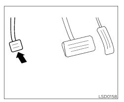
**To engage:** Firmly depress the parking brake.
