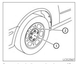
Removing bolt-on wheel caps (if so equipped)
