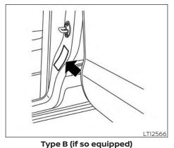
The cold tire pressure is shown on the Tire and Loading Information label. The label is located as shown.
