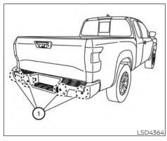
The RAB system detects obstacles behind the vehicle using the parking sensors (1) located on the rear bumper.
