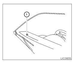
Be sure you do not put anything on top of the autolight sensor ① located in the top side of the instrument panel. The autolight sensor controls the autolight; if it is covered, the autolight sensor reacts as if it is dark out and the headlights will illuminate. If this occurs while parked with the engine off and the switch in the ON position, your vehicle's battery could become discharged.
