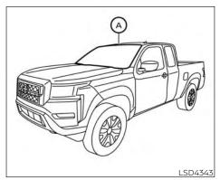
The TSR system provides the driver with information about the most recently detected speed limit. The system captures the road sign information with the multisensing front camera unit (a) located on the windshield in front of the inside rearview mirror and displays the detected signs in the vehicle information display. For vehicles equipped with a navigation system, the speed limit displayed is based on a combination of navigation. TSR information is always displayed at the top of the
