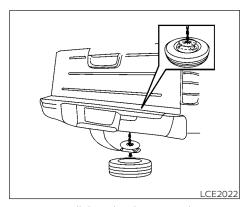
3. To reinstall the wheel, remove the center cap and insert the tire chain through the wheel. Be sure the rubber spacer is centered on the wheel before lifting. Use the assembled jacking rod to slowly rotate the winch clockwise to raise the wheel to the vehicle.
