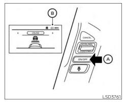
Operating vehicle-to-vehicle distance control mode
