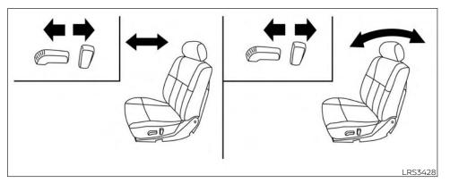
The reclining feature allows adjustment of the seatback for occupants of different sizes for added comfort and to help obtain proper seat belt fit. For additional information, see "Precautions on seat belt usage" (P. 1-15). Also, the seatback can be reclined to allow occupants to rest when the vehicle is stopped and the shift lever is in P (Park) or N (Neutral) position with the parking brake fully applied.
