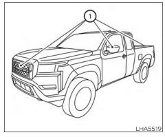
To display the multiple views, the Intelligent Around View Monitor system uses cameras located in the front grille, on the vehicle's outside mirrors and one on the tailgate 1).
