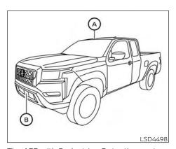
The AEB with Pedestrian Detection system uses a radar sensor located on the front of the vehicle (B) to measure the distance to the vehicle ahead in the same lane. For pedestrians, the AEB with Pedestrian Detection system uses a camera installed behind the windshield (A) in addition to the radar sensor
