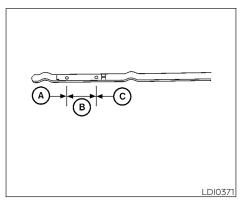
5. Remove the dipstick again and check the oil level. It should be between the H (High) and L (Low) marks (a). This is the normal operating oil level range. If the oil level is below the L (Low) mark (a), remove the oil filler cap and pour recommended oil through the opening. **Do not overfill** (a).
