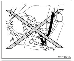
Even with the NISSAN Advanced Air Bag System, never install a rearfacing child restraint in the front seat. An inflating front air bag could seriously injure or kill your child. For additional information, see "Child restraints" in this section.
