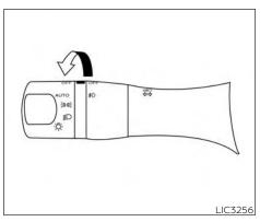
The headlights must be on and the low beams selected for the fog lights to operate. The fog lights automatically turn off when the high beam headlights are selected.
