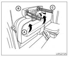
1. To access the jump seat extension (passenger's side only) (A) on the jump seat, pull up (B) on the extension to unfold it to the open position. Then unfold the two support legs (and lower the jump seat to the full open seating position.
