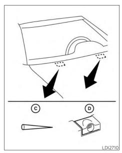
Be careful not to let anything get into the washer nozzle (1). This may cause clogging or improper windshield-washer operation. If something gets into the nozzle, remove it with a needle or small pin (3)
