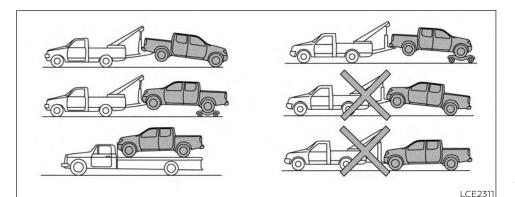
Two-Wheel Drive models with automatic transmission
