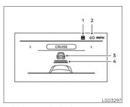
Vehicle-to-vehicle distance control mode display and indicators
