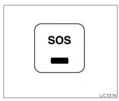
The Emergency call (SOS) system button is combination with used NissanConnect® Services subscription to call for assistance in case of an emergency.
