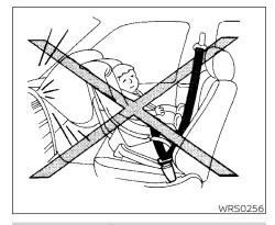
Even with the NISSAN Advanced Air Bag System, never install a rearfacing child restraint in the front seat. An inflating front air bag could seriously injure or kill your child. For additional information, see "Child restraints" (P. 1-28).
