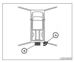
When the corner of the vehicle moves closer to an object, the corner sonar indicator  ${\Large \textcircled{\sc A}}$  appears. When the center of the vehicle moves close to an object, the center sonar indicator (B) appears.
