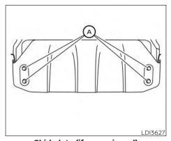
Skid plate (if so equipped) Removal of under-engine protectors
