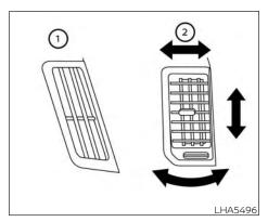
Adjust air flow direction for the driver and passenger's side vents or center vents (2) by moving the vent slide and/or vent assemblies. Open or close the driver, passenger and center vents by using the dial. The defrost vents (1) located above the driver and passenger side vents cannot be adiusted or closed.
