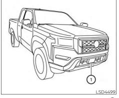
The I-FCW system uses a radar sensor (1) located on the front of the vehicle to measure the distance to the vehicle ahead in the same lane.
