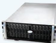
CSE-947SE1C-R1K66JBOD 60x 3.5" 4U Top Loading SAS/SATA 12Gb/s Hot Swapping HHD/SSD
