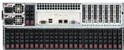
SC417BE2C/E1C-R1K28LPB Rear view With 24x 2.5" HDDs
