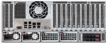
SC846X Rear View (13 FH/FL slots), BBP® Support
