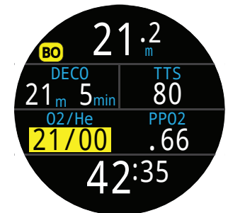
14. Gas Switch Required
